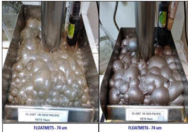
Figure 1. Froth Formation for Silver Extraction from Transition and Sulphide Materials
